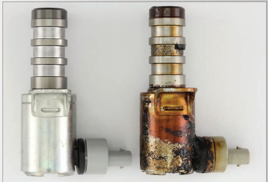
As motor oil degrades, sludge and varnish can cause VVT solenoids to stick or malfunction, leading to poor engine performance or even damage.
