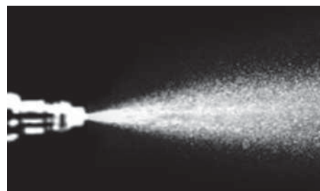
Injector spray pattern after P.i. treatment.
